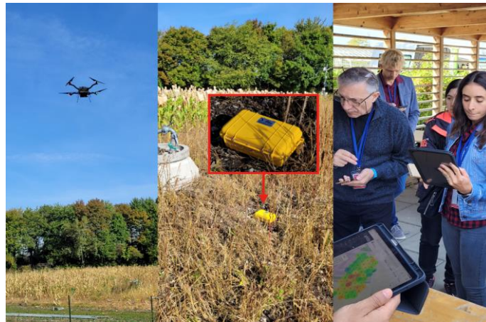
The UAV technology utilizes quadcopter with plastic scintillation detector to quickly scan a large area where the mapping data and progress can be monitored from a safe location.
