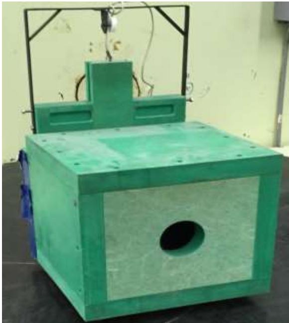
Figure 6: Irradiation Box (Boron Polyethylene)
