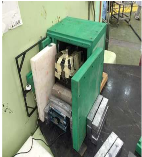
Figure 7. Experimental Neutron Spectrometer Set-up
