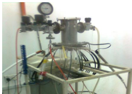
Dense plasma focus (DPF) device of Mather type at Malaysian Nuclear Agency
